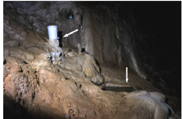
Figure 4. Drip pool 5 in Škocjanske jame modified to be a permanent water source. Arrows indicate the drip with a filtration unit underneath and the pool, offset from the drip.
