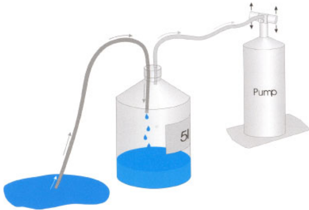
Figure 2. Apparatus for aspirating water in pools. After aspiration, the water and sediment mixture in the container is passed through a filtering bottle for preservation.
